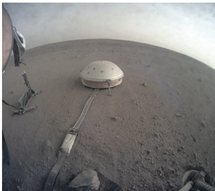
This April 25, 2019 photo made available by NASA shows the InSight lander's dome-covered seismometer, known as SEIS, on Mars. On Tuesday, Oct. 1, 2019, scientists released an audio sampling of marsquakes and other sounds recorded by the probe.
